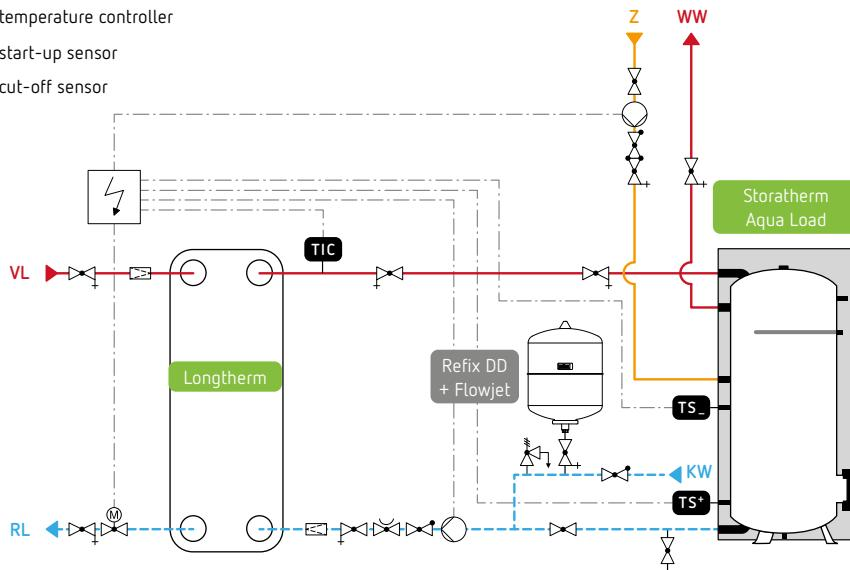
Select a potable water outlet temperature  $\leq 60^\circ\text{C}$  if possible, to minimise the risk of calcification (heating medium temperature  $\leq 70^\circ\text{C}$ ). For a continuous through flow on the potable water side, the calcification risk is lower; if necessary, incorporate the circulation line on the cold water side after the charging pump.
