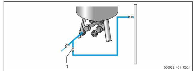
Preferably use a water hose to fill the primary vessel with water when the automatic make-up device is not yet connected.
