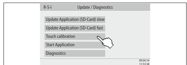
You can calibrate the touch screen when touching the desired buttons does not work satisfactorily.
