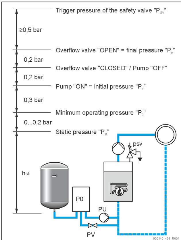
The "P<sub>0</sub>" minimum operating pressure is calculated as follows:
