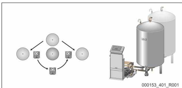
Determine the positions for the control unit, primary vessels and secondary vessels (if used).
