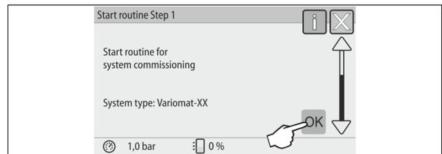
The system automatically displays the first page of the start routine when you switch on the device for the first time:
