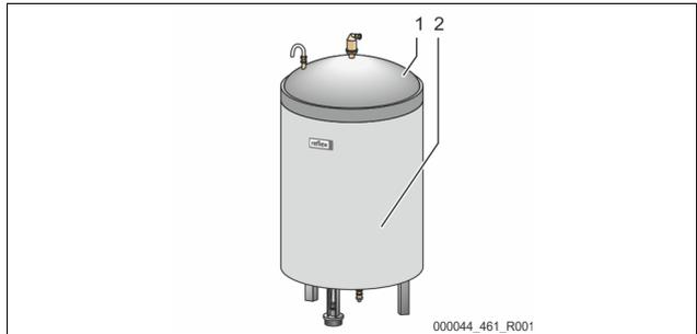
Install the optional thermal insulation (2) around the primary tank (1) and close the insulation with the zip fastener.
